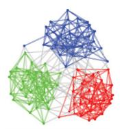
(b) A good edge-cut of the same graph, where vertices that are highly connected are assigned to the same partition.
