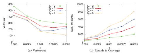
Fig. 8. Tuning simulated annealing parameters on data graph from Walshaw archive (K = 2).
