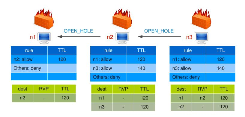
Through this chain n3 can shuffle with n1.
