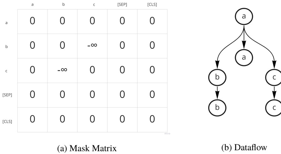
Figure 3.5: Graph-Guided Masked Attention’s mask matrix (Left) on an example data flow (Right).
