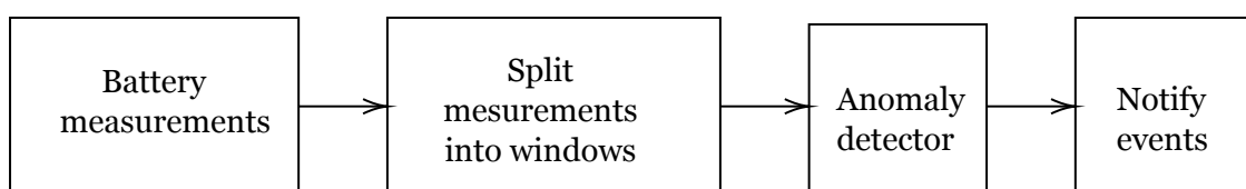
Figure 4.1.1: The high-level concept of battery anomaly detection.
